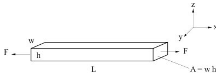
Figure 2.1 A long slender bar with an axial load.
