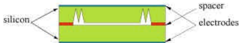
Figure 3.3 Bulk-micromachined capacitive pressure sensor with silicon substrate.
