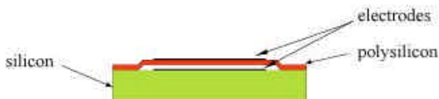
Figure 3.4 Surface-micromachined capacitive pressure sensor.
