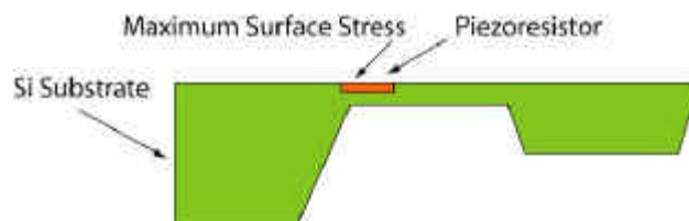
Figure 1.3 Cantilever beam sensor with piezoresistive gauge.
